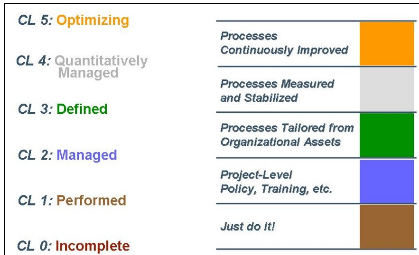
Figure 2—Capability Levels (CL) for Risk Management in the CMMI RSKM Process Area
